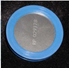
FRM sampler Delrin 47mm filter holder ring with stainless steel grid
