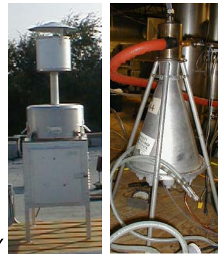
Dual Channel Sequential Filter Sampler and Sequential Gas Sampler Desert Research Institute, Reno, NV
