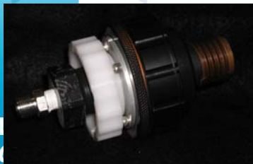
Speciation sampler Teflon-coated aluminum filter holder
