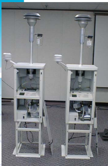
Mass Aerosol Sampling System (MASS) URG Corporation, Raleigh, NC
