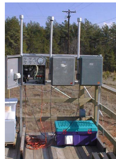
Interagency Monitoring of Protected Visual Environments (IMPROVE) Sampler Air Resource Specialists, Ft. Collins, CO
