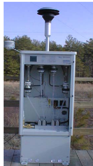
Reference Ambient Air Sampler (RAAS) Andersen Instruments, Smyrna, GA
