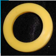
Dichotomous sampler polyethylene 37mm filter holder
