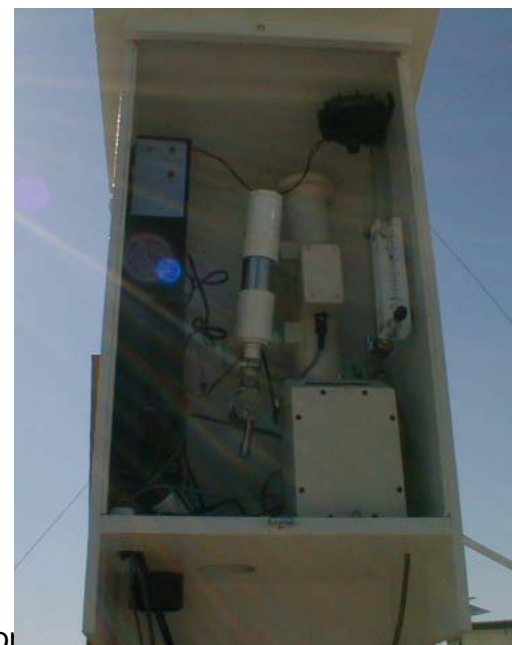
Radiance M903 nephelometer with smart heater
