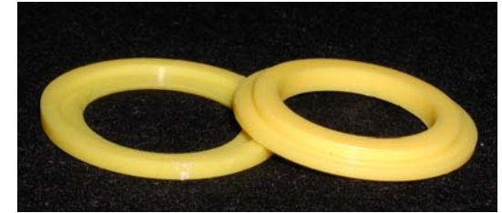
Dichotomous sampler polyethylene 37mm filter holder
